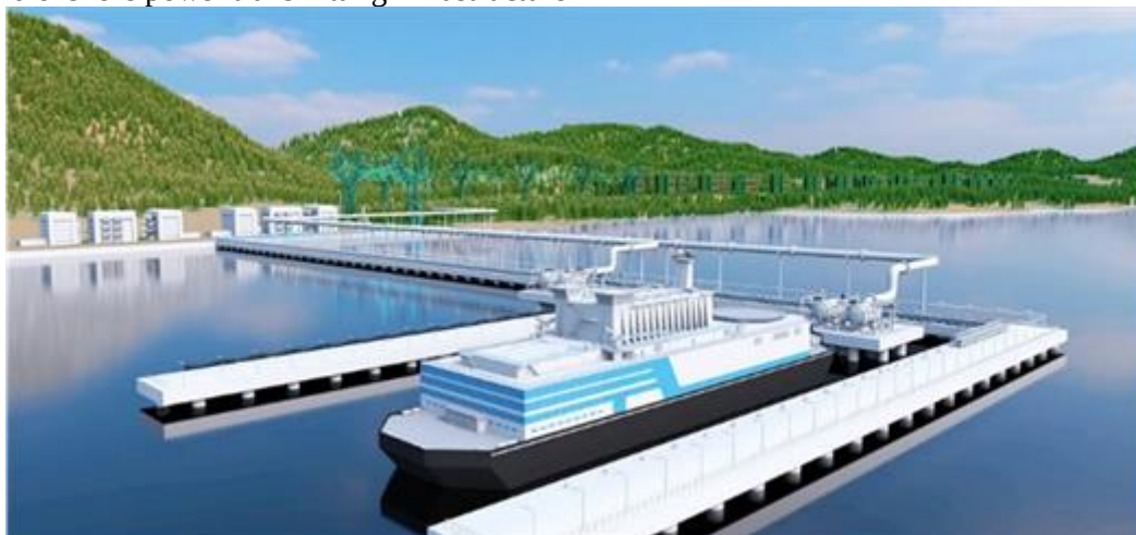
OFPU fitted with the RITM-200M reactor plant
