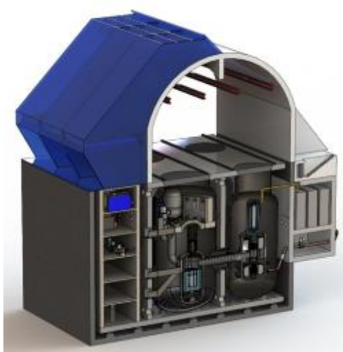
Elevation view of EM 2 modular building element employing two modules on a single seismically isolated platform
