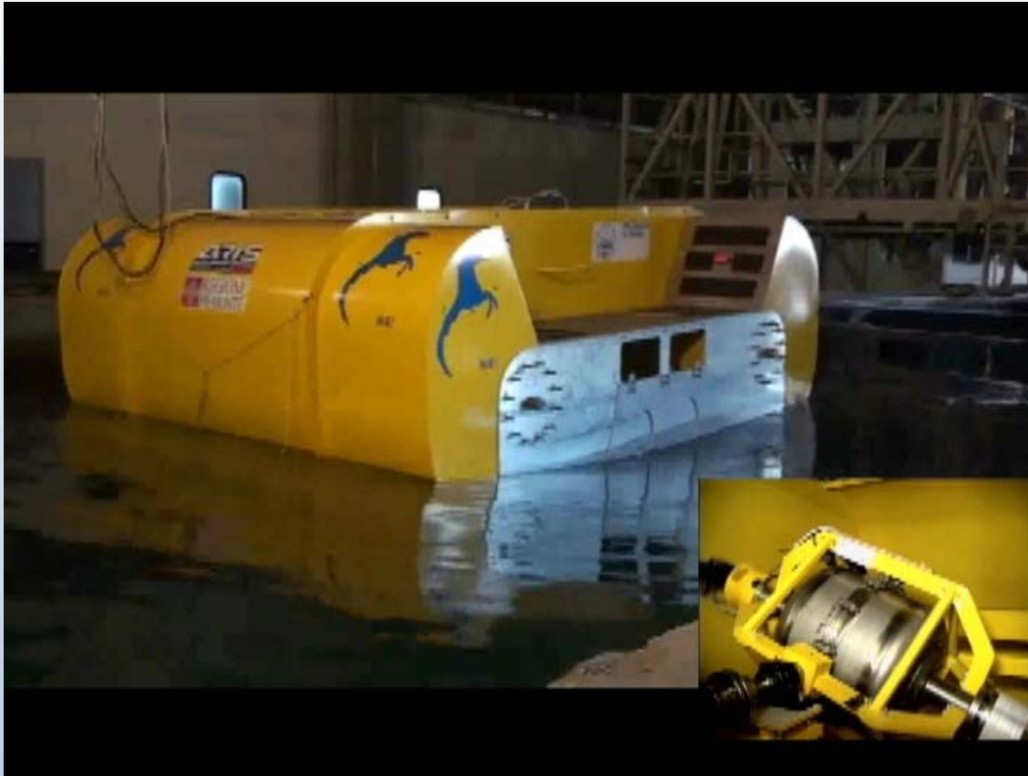
1:8 Prototype tank test CNR-INSEAN Wave Tank
