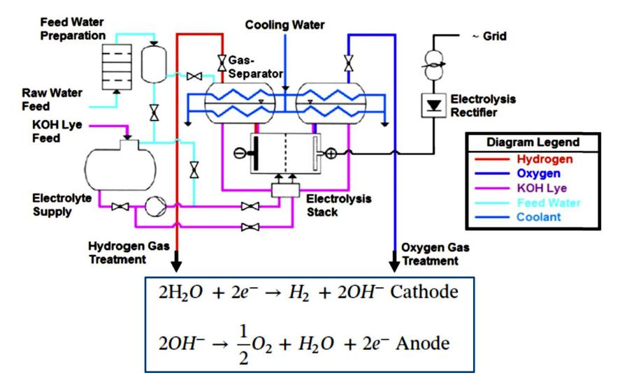
Alkaline Electrolysers not suitable for electricity dispatching, because of high transients <sup>3</sup>
