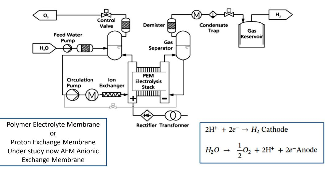
PEM higher current density, efficiencies and modulation capacity, but higher costs, low pressure, membrane technology
